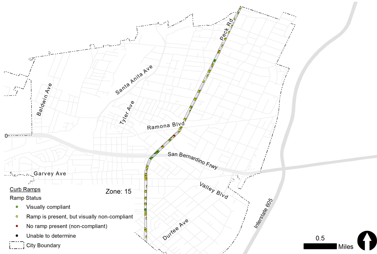
FIGURE C-15: Zone 15 Curb Ramps
